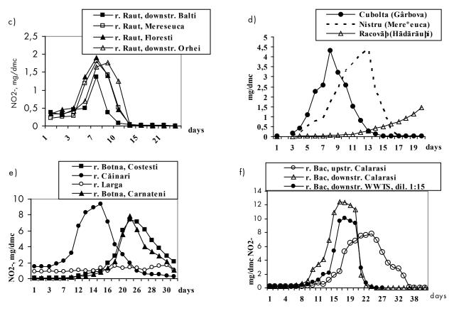
Figure 2. Evolution of the second stage of nitrification  $(NO_2^- \rightarrow NO_3^-)$  in rivers water.
